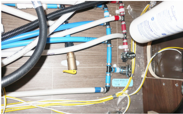
Waterlines and Tank Drain Valves *Model 59K shown (See “Water System Drain Valve Locations” chart at the end of this section for location on your model)
