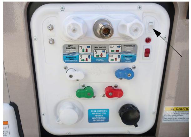
Water pump switch location on Water Center Panel *Model 59K shown -Typical View
