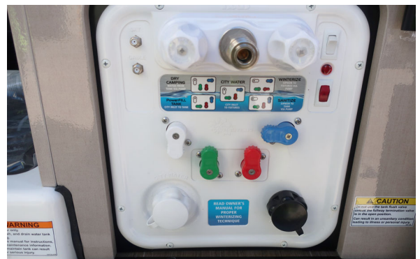
Exterior Shower/Wash Station (Located behind rear passenger side door on the 59K, and behind the drivers rear door on the 59G.) *Model 59K shown - Typical View
