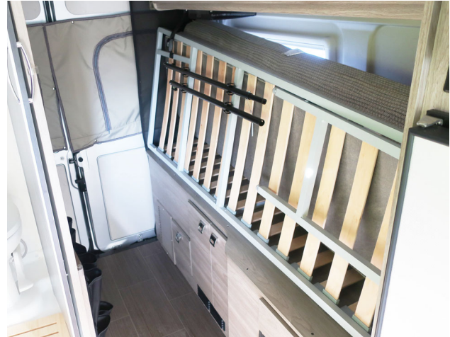
The bed is located on the drivers side rear, folded up and locked with a seatbelt for storage. -Typical View
