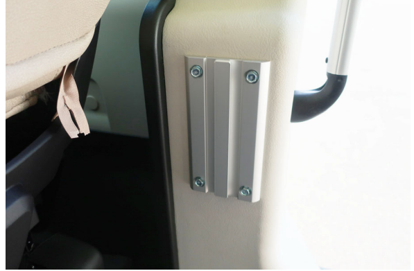
The second dinette table attachment point is located inside the passengers wall next to the main entry door. -Typical View
