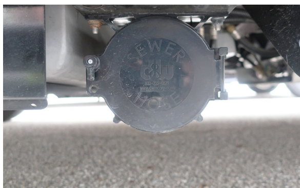
Sewage Drain Hose (Located beneath left sidewall) -Typical View
