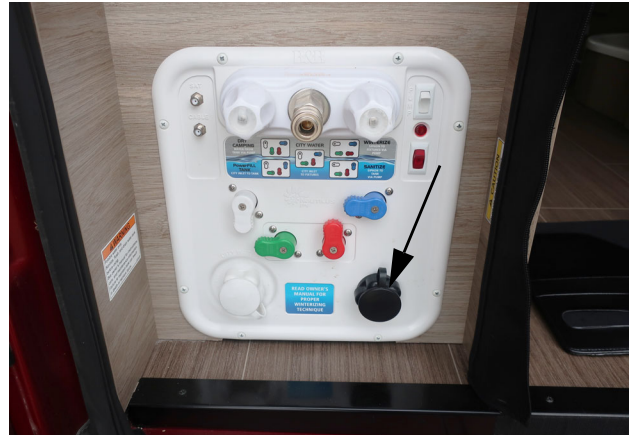
Black Waste Tank Flush Inlet (Located on Water Center Panel) -Typical View
