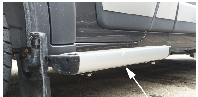
Accent LED Light Strips (Located on driver side running board) -Typical View
